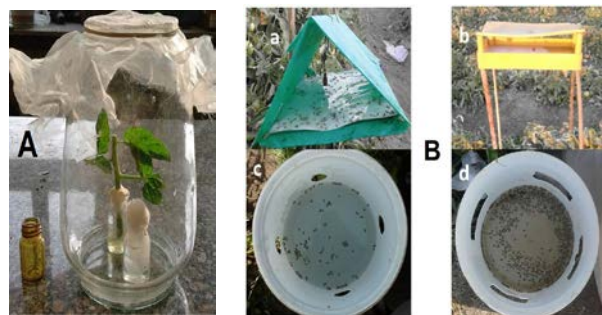
Fig. 1. A- Adult rearing chimney cage; B- traps types contains (a- sticky delta trap; b- water pan trap; c- palm weevil bucket trap; d- modified palm weevil bucket trap).
